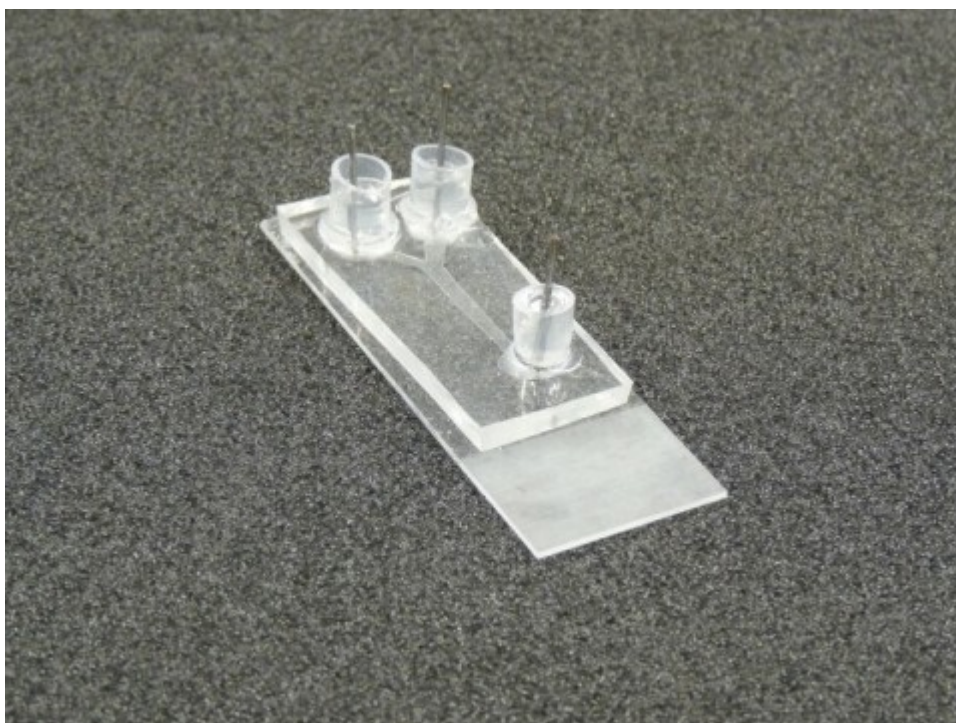
Figure 7: Stable connectors for tubing as described in Chips&Tips
