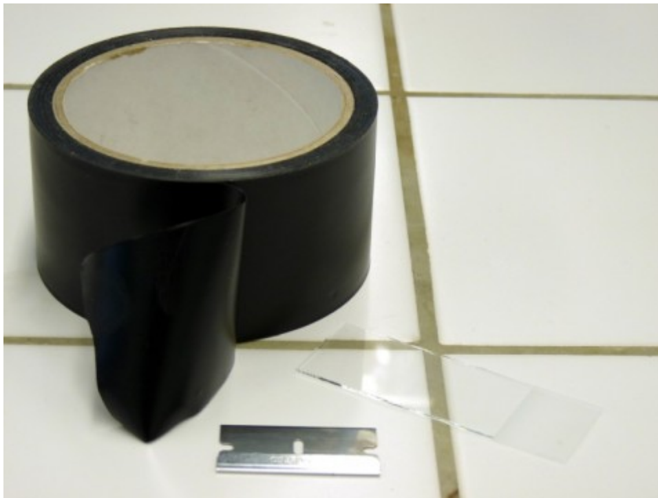
Figure 1: material needed: tape, a rozorblade/cutting knife, a glass slide and PDMS
