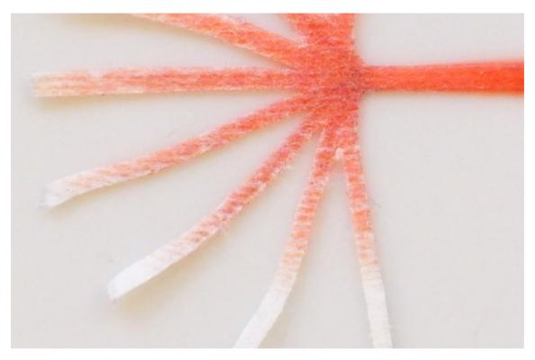
The speed of fluid flow in paper microfluidic channels can be controlled by cutting paper at different angles to the paper grain. Fluid in the the central branch cut parallel to the grain has reached the end, while in the vertical branches cut perpendicular to the grain it has not yet.
